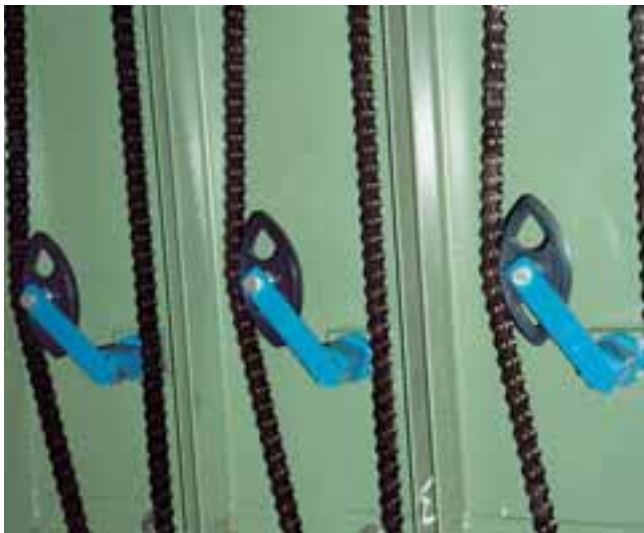
Chain tensioner with glider on processing machine
