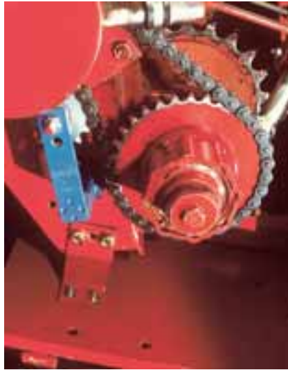
Chain tensioner on baling press
