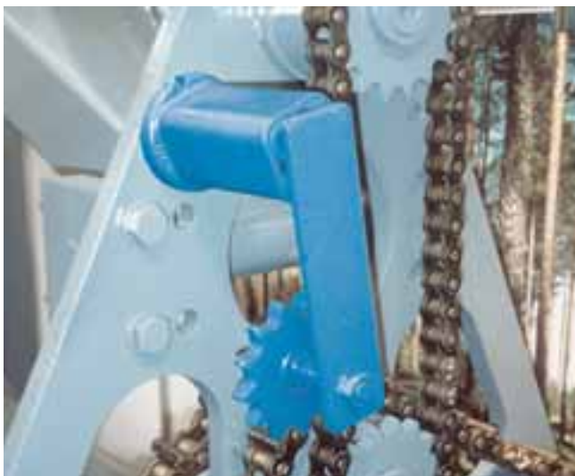
Chain tensioner on paper rolling mechanism
