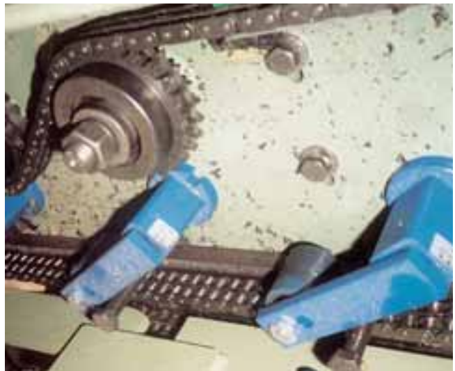
Elastic chain guidance on wood intake
