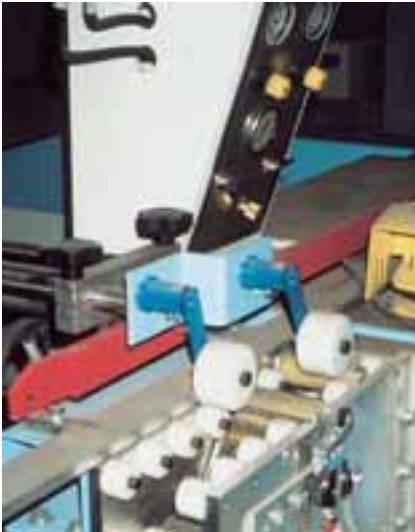
Suspension of tensioning rollers on a wrapping machine
